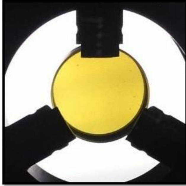
Figure 5.6.5: Sample B15-5 after a total of 96 hours of exposure to high intensity UV light, resulting, in an transmission value at 792 nm of 89.33%.
